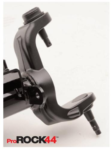
One of the best features of the New ProRock 44 is the new, stronger end forging. This forging is 100% Made in the USA. It is a true steel forging, and not a cheap casting. This forging, the high ground clearance housing, and the big 3.0" (77mm) diameter tubing will prevent the bending problems which are common on the stock JK housings.
